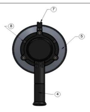
Figure 2: Flame Simulator Rear View
